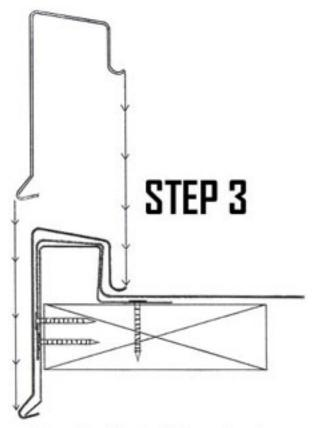
SNAP FASCIA SECTION DOWN INPLACE MAKING SURE THE DRIP EDGE ENGAGES THE CANT DAM. YOU MUST ALSO APPLY THE SPLICE PLATE AT THIS POINT. LEAVE AT LEAST 1/4 GAP FOR EXPANSION.
