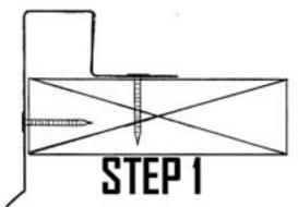
NAIL A CONTINUOUS GALVANIZED CANT DAM TO AN APPROVED NAILER BY USING A 1 1/4 GALVANIZED NAIL. NAILS SHOULD BE 12" ON CENTER AND THERE SHOULD BE A 3/16 GAP BETWEEN THE CANT DAM FOR EXPANSION.
